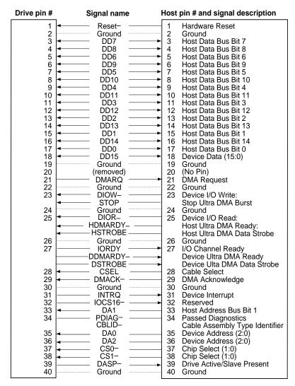
Pins 28, 34 and 39 are used for master-slave communication (details shown below).
