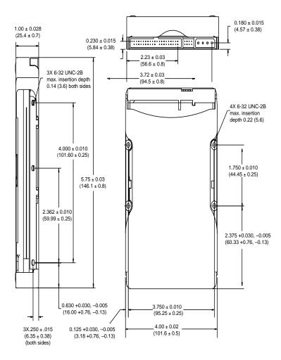
Figure 3. Mounting dimensions—top, side and end view
